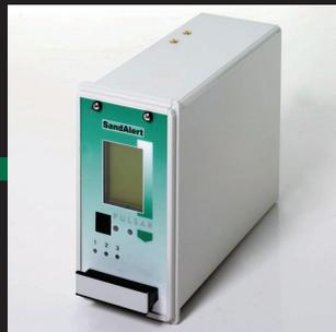
In panel mount guise, SandAlert is designed for mounting on a control panel where front panel space may be at a premium. All wiring is conveniently accessible from the rear of the panel mount enclosure and the electronics may be removed without disturbing the wiring connections or compromising the safety or integrity of the installation. Programming is via the optional Pulsar hand-held infra red programmer or RS232 PC link.
