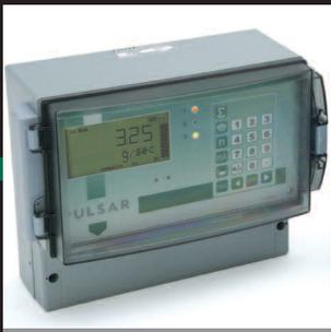
SandAlert in its Wall Mount format is typically used in single point fixed and semi-permanent installations. This version features a polycarbonate enclosure to IP65. Programming the unit is simple using the integral membrane keypad or via RS232 connection from a PC.
