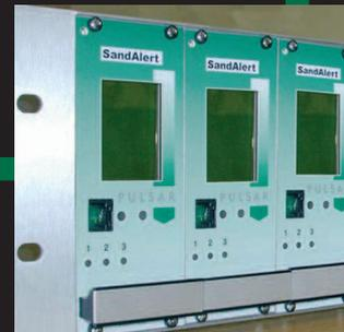
The 19" rack mounted version of the SandAlert lends itself perfectly to multipoint installation. Each unit is 3U high and 10HP wide and features a back-lit LCD display showing a bar graph and an instant readout of sand mass.
